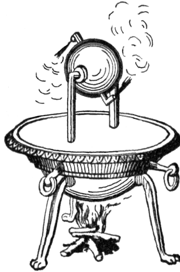
Figure 3.1: Illustration of the Hero's steam engine [2]
