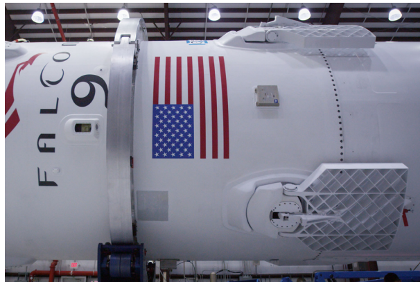
Figure 4.2: Grid fins on the Falcon 9 rocket [8]
